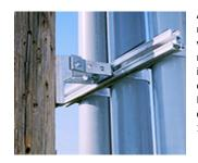
A multi-purpose bracket for mounting 1" thru 6" conduit in a variety of ways. This bracket will mount up to six 6" conduits with infinite adjustability. 4-Way T-Slot extrusion eliminates field drilling. Mounts to the pole on 3 5/8" hole centers with 5/8" thru bolt and 1/2" lag screws (not supplied).
